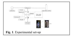
The continuous gas-liquid flowing film reactor used in this study, shown in Fig. 1, is like that used in previous work [2]. Argon was used as the carrier gas and DI water was used as the liquid phase. DI water was supplied to the system with high-pressure reciprocating pump at 2mL/min.
